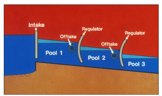
In each pool, the water level should remain within a maximum and minimum level but the surface profile can take any position within the two extreme lines.
