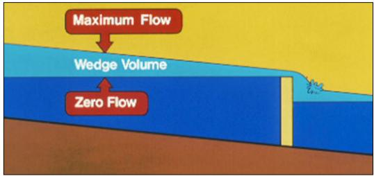
In other words, the basic design of an irrigation system operated continually with variable flows is to divide the canals into successive pools and to locate the regulators and the off-takes in such a way that the differential water level variations remain within certain limits.
