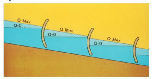
If the cross regulators are manually operated, each one should be adjusted at frequent intervals as the flow change moves downstream. Many small adjustments may be necessary because the change in flow rate arrives gradually at various regulators. It is difficult to make predictions of the necessary adjustments in control gates because of the large number of hydraulic variables. It is almost impossible to set the flow released at the head regulator of the branch
