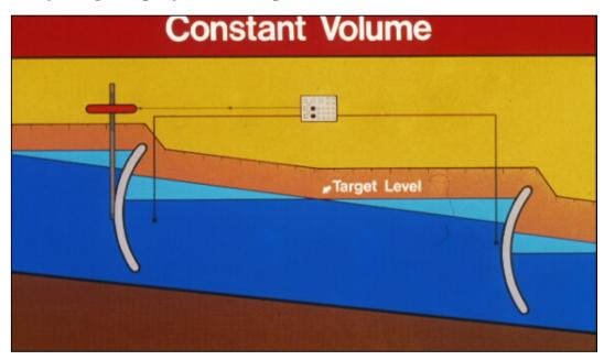
The target level in any section could also be between two regulators. When the control point is approximately in the middle of a pool, this method is called constant volume.
